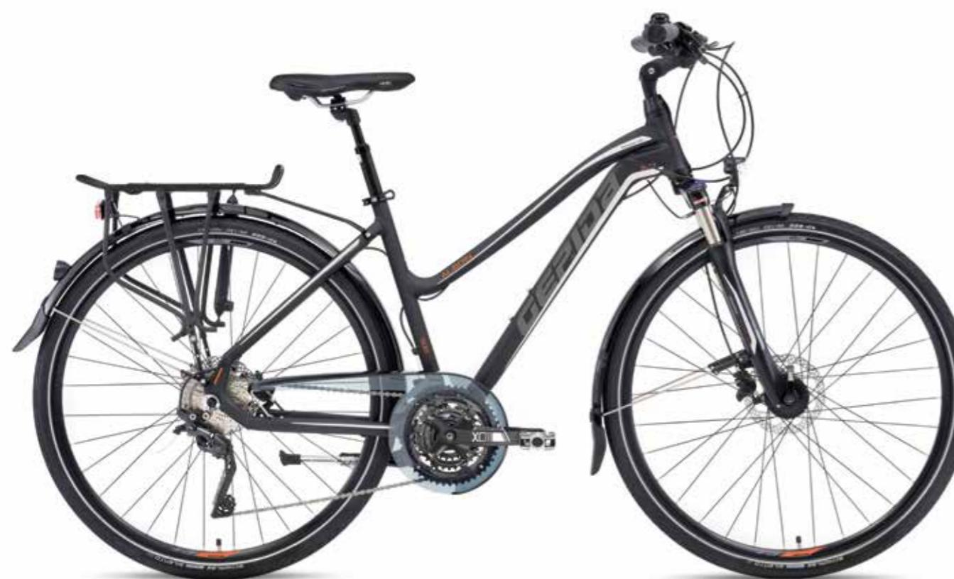
△ FRAME GEPIDA HYDROFORMING - 6061 ALLOY
