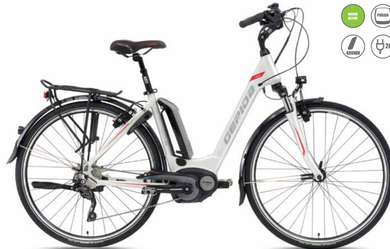
△ FRAME GEPIDA HYDROFORMING - 6061 ALLOY
