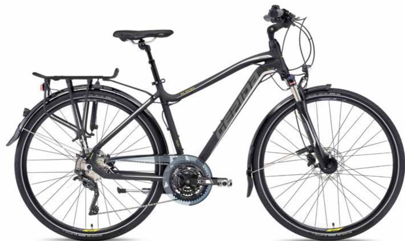
△ FRAME GEPIDA HYDROFORMING - 6061 ALLOY
