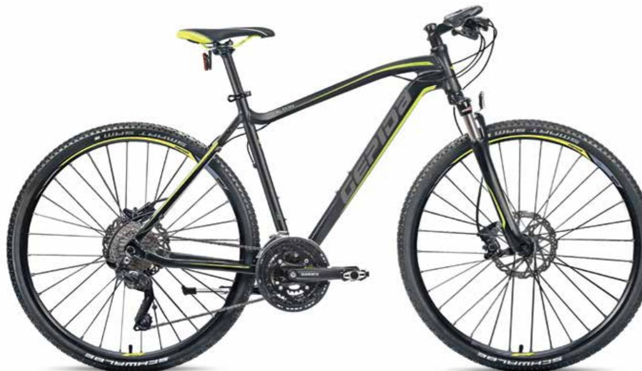
△ FRAME GEPIDA HYDROFORMING - 6061 ALLOY
