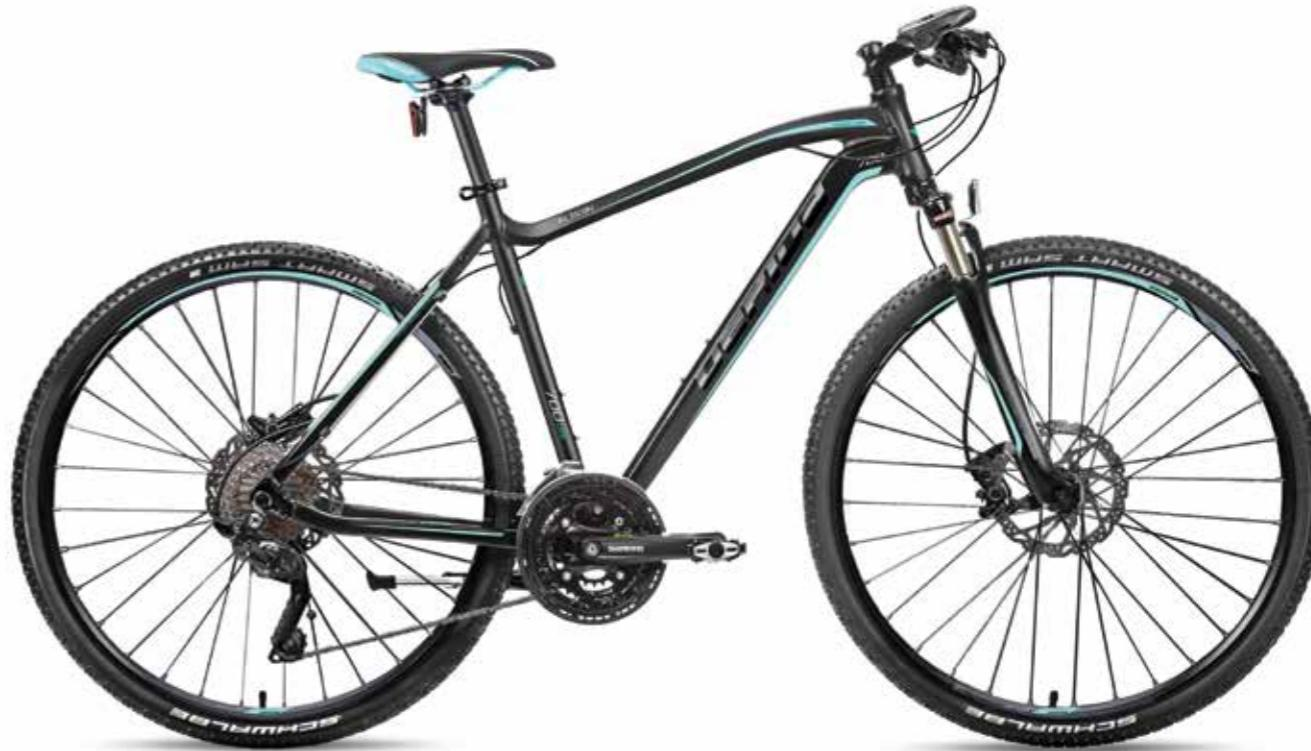
△ FRAME GEPIDA HYDROFORMING - 6061 ALLOY
