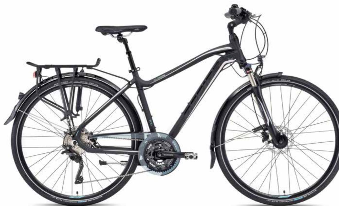
△ FRAME GEPIDA HYDROFORMING - 6061 ALLOY
