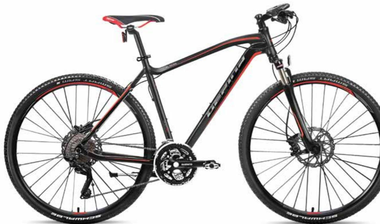
△ FRAME GEPIDA HYDROFORMING - 6061 ALLOY
