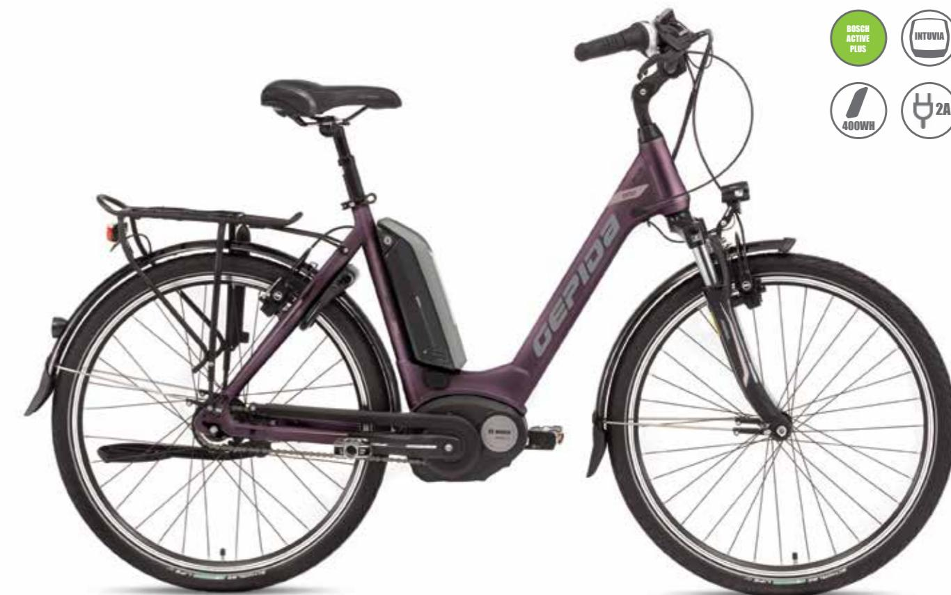
△ FRAME GEPIDA HYDROFORMING - 6061 ALLOY
