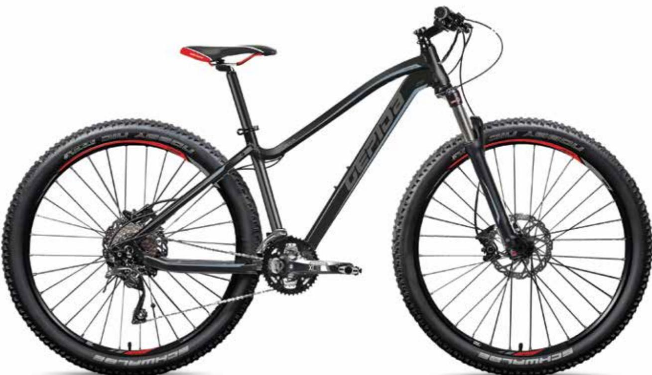
△ FRAME GEPIDA HYDROFORMING - 6061 ALLOY
