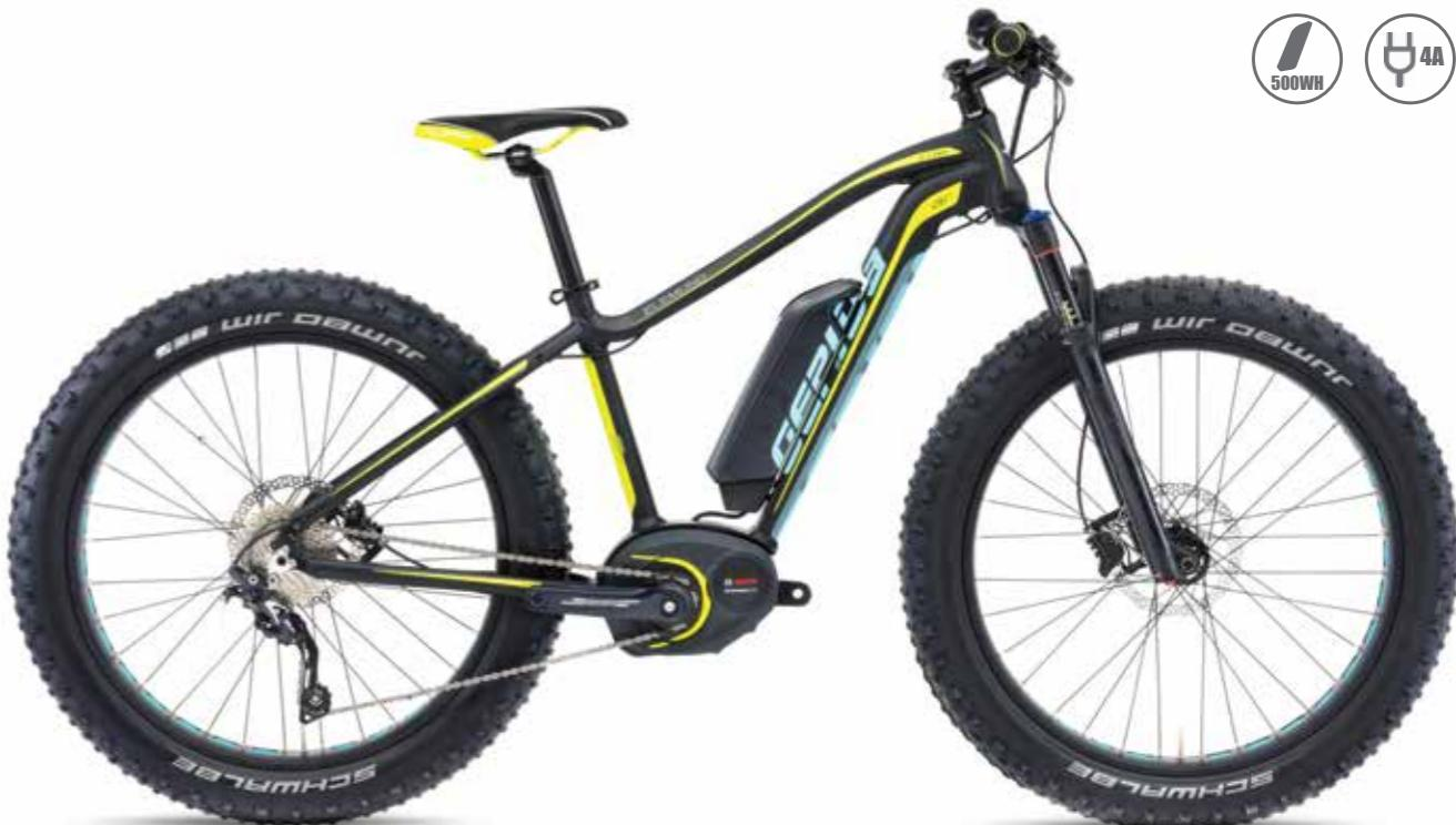
☐ FRAME GEPIDA HYDROFORMING - 6061 ALLOY
