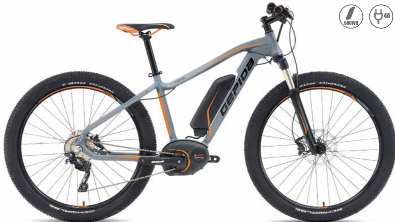
△ FRAME GEPIDA HYDROFORMING - 6061 ALLOY
