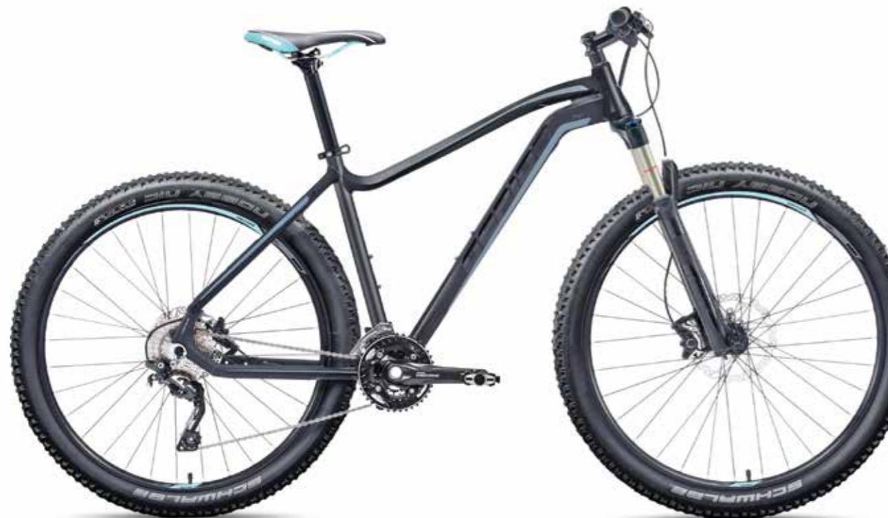
△ FRAME GEPIDA HYDROFORMING - 6061 ALLOY
